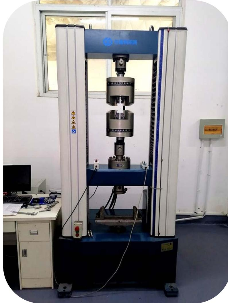
Mechanical tensile tester
