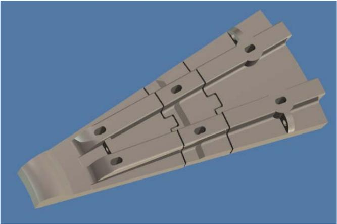
Segment design according to different abrasion degree
