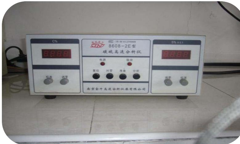
Carbon sulfur analyzer
