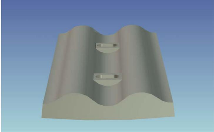
Double wave crest design of overflow mill liner
