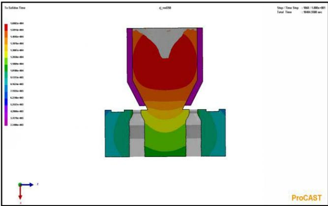
Liner optimization through multiple simulation of casting process.
